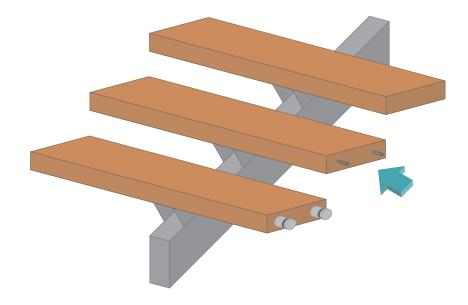
Situation 2: Wood to be installed around the metal plates using thinner wood planks.
