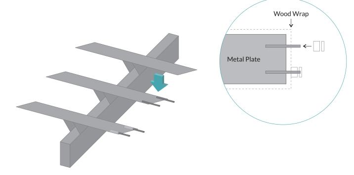
Excess bolt (outside) can be cut later if necessary.
